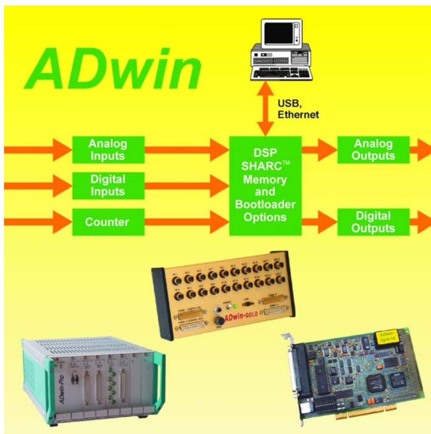
Fig. 1 – Concept of the ADwin systems
