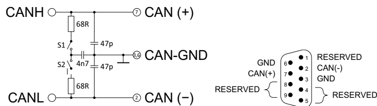
Fig. 147 – Pro II-CAN-FD-2 Rev. E: Block diagram and pin assignment (male)
