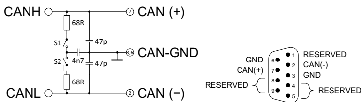
Fig. 150 – Pro II-CAN-FD-2 Rev. E: Block diagram and pin assignment (male)
